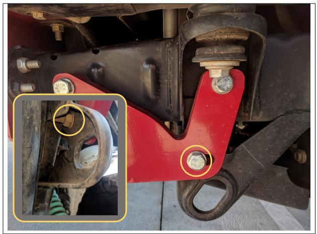
8. On LHS fit extra M12x65 Bolt, using the M12 Flange nut behind the factory tie down point as shown.
