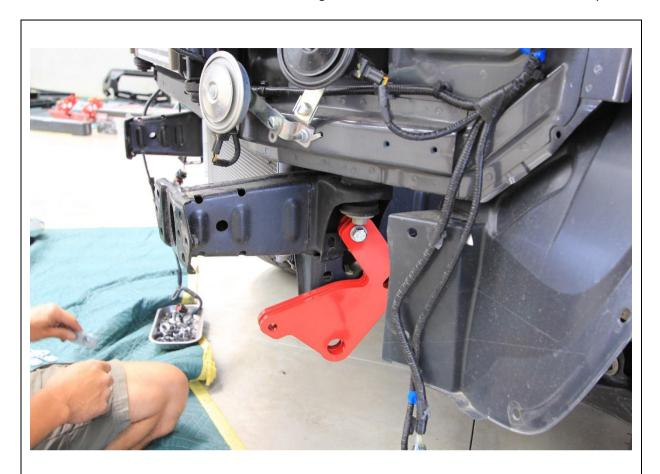
5. Place tow points onto chassis rail and insert bolts into holes.
